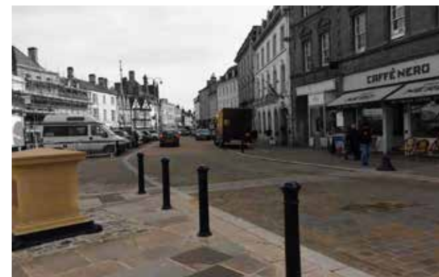
Figure 6: Positive example of two streets in Cirencester, where the use of materials and vertical deflection, provide a pedestrian priority environment and is aesthetically pleasing.
