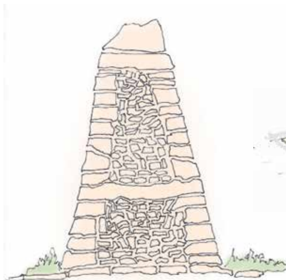
Figure 43: Example showing the construction of dry-stone wall.
